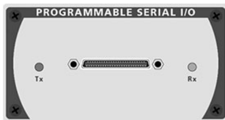
This illustration shows the Programmable Serial module and Programmable Serial Pod.
