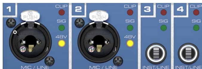
Figure 3. A portion of the front panel of an RME Fireface UC audio interface showing XLR combo jacks (1-2) and TRS jacks (3-4)
